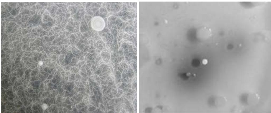
Figure 1. Bacteria and actinomycetes in non-contaminated (left) and hydrocarbon-contaminated soil (right)– Icoana
