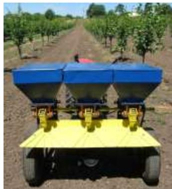
Fig. 4 **Granular solid fertilizer delivery equipment:**
