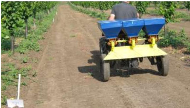
Fig.6 Gravitational use of fertilizers
