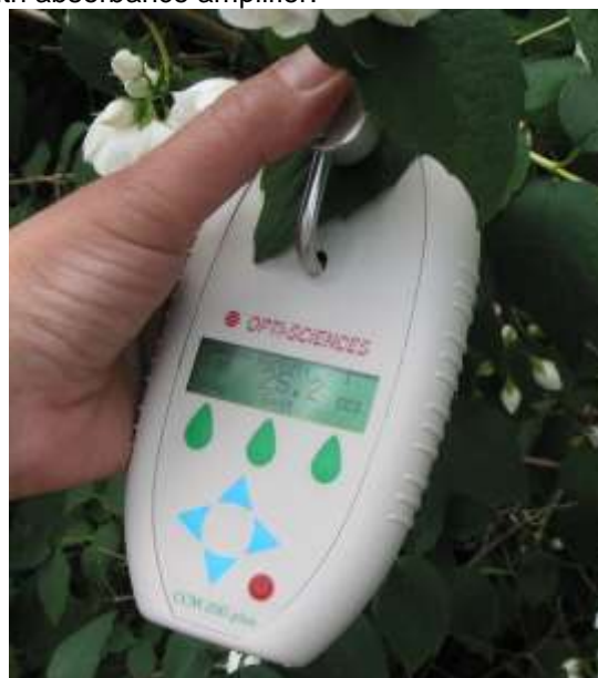
Figure1 Device used for determining the chlorophyll content of leaves ( http://www.marconi.com.br )
