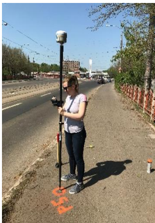
Figure 3 a) GPS Stonex S8 measurements b) Stationing with level on control point P6 c) Classical level Carl Zeiss Ni 002
