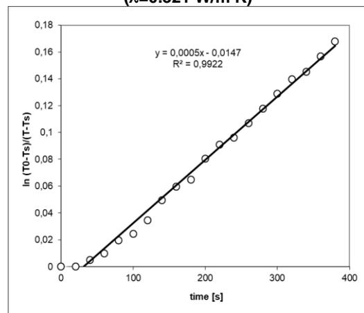
Figure 7 Experimental results for Transylvanian salami ( $\lambda=0.243$  W/m·K)
