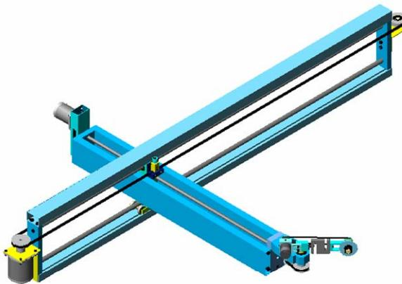
**Fig. 2 - Manipulator PPR with 3 DOF**
