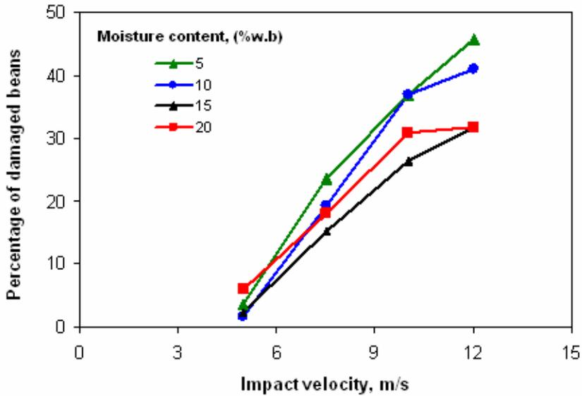
Fig. 2 - Effects of impact velocity on the percentage of physical damage in kidney beans
