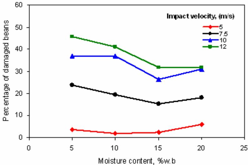
**Fig. 4 - Effects of moisture content on the percentage of the physical damage in kidney beans**
