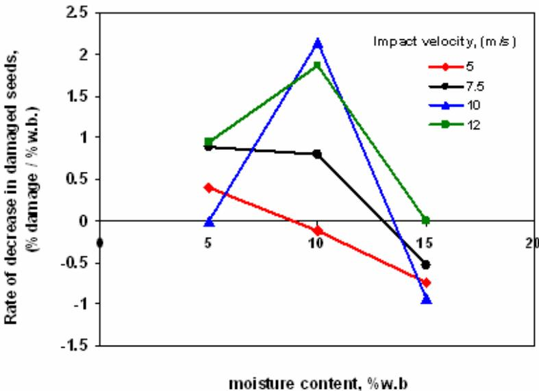
Fig. 5 - Rate of increase in the physical damages of kidney beans versus moisture content
