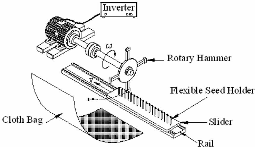
Fig. 1 - Schematic diagram of the impact device used in this study
