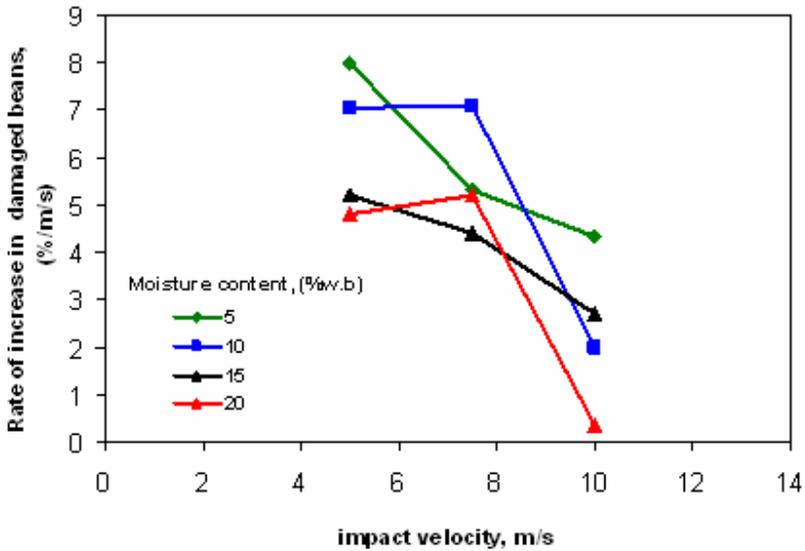
Fig. 3 - Rate of increase in physical damages of kidney beans versus impact velocity
