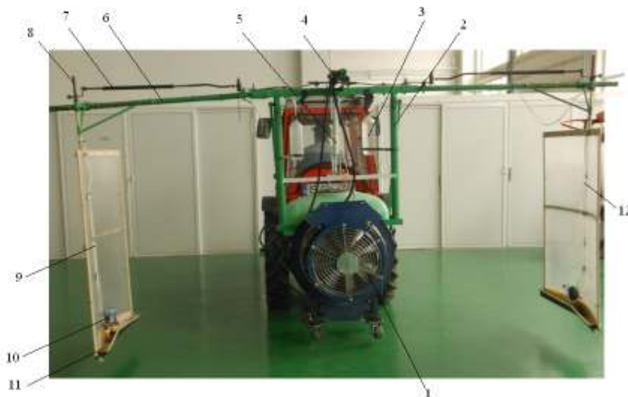
Fig. 1 - Sprayer unit with equipment for recovering sprayed solution: 1 - car splashes; 2 - the metal frame; 3 - graduated cylinders; 4 - hydraulic cylinder; 5 - thrusts; 6 - collapsible support; 7 - parallelogram mechanism; 8 - rods; 9:12 - panels; 10 - pumps; 11 - gutters.
