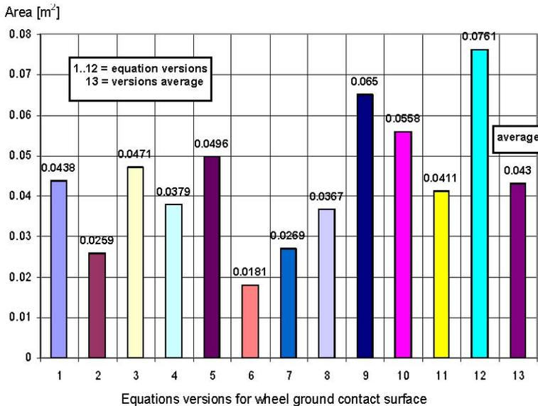
**Figure 1 - Wheel-soil contact surface for different kinds of equations regarding this area (the U-650 tractor, front wheel)**
