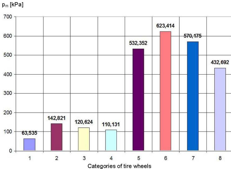
**Figure 6 - Average wheel-soil pressure:**
