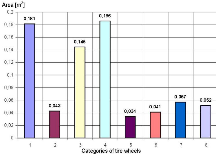
**Figure 5 - Average wheel-soil contact patch area:** 1 – U-650 tractor (rear wheel); 2 –U-650 tractor (front wheel); 3 – Valtra T-190 tractor (front wheel); 4 – Valtra T-190 tractor (rear wheel); 5 – 5 tonnes 2RB5AT trailer (wheel); 6 – 7 tonnes 7RBAT trailer (wheel); 7 – large dump capability Iveco Trakker 8x4 P<sub>1</sub> and P<sub>2</sub> axle (wheel); 8 – large dump capability Iveco Trakker 8x4 P<sub>3</sub> and P<sub>4</sub> axle (wheel).
