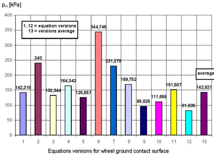
**Figure 2 - The average pressure exerted by the wheel on the ground for different versions of wheel-ground surfaces equations (the U-650 tractor, front wheel)**
