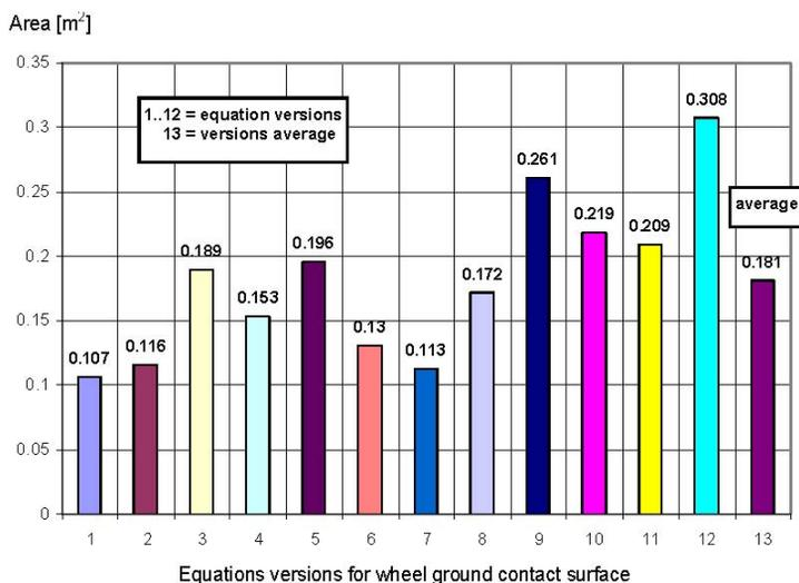
**Figure 3 - Wheel-soil contact surface for different kinds of equations regarding this area (the U-650 tractor, rear wheel)**
