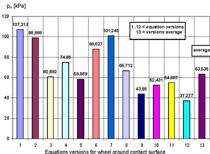
**Figure 4 - The average pressure exerted by the wheel on the ground for different versions of wheel-ground surfaces equations (the U-650 tractor, rear wheel)**
