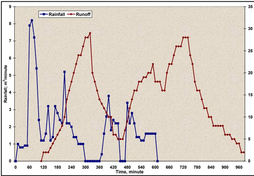
Figure 2- Runoff (l/minute) hydrograph, on August 5, 1987, in Scobâlțeni watershed
