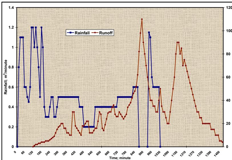
Figure 5 - Runoff (l/minute) hydrograph, on September 7, 1989, in Scobâlteni watershed
