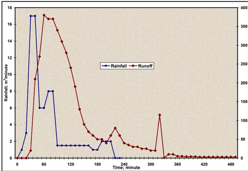
Figure 4 - Runoff (l/minute) hydrograph, on August 15, 1989, in Scobâlteni watershed
