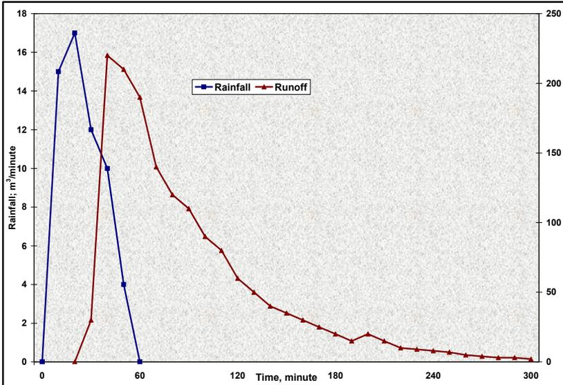
Figure 3- Runoff (l/minute) hydrograph, on June 25, 1989, in Scobâlțeni watershed
