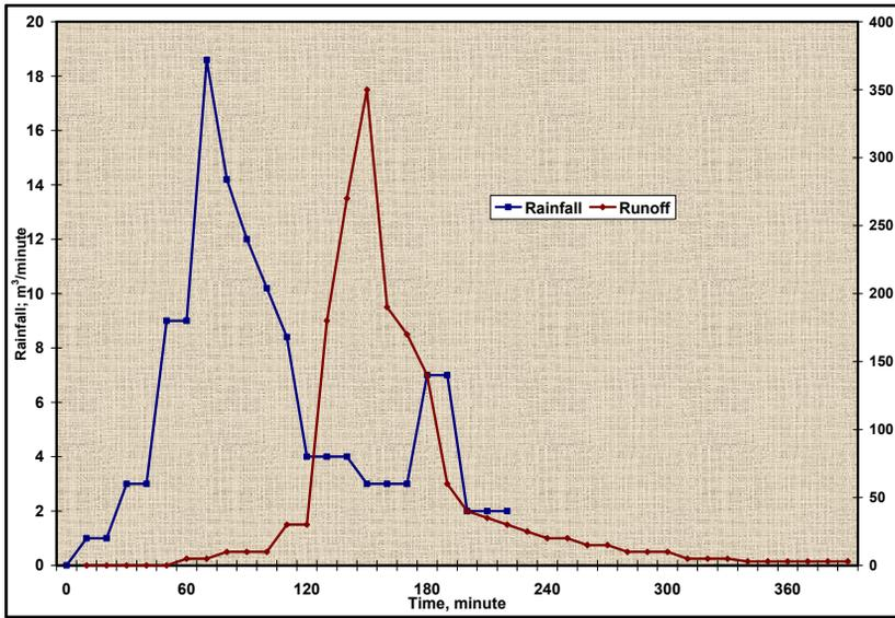
Figure 6 - Runoff (l/minute) hydrograph, on July 1, 2006, in Scobâlteni watershed
