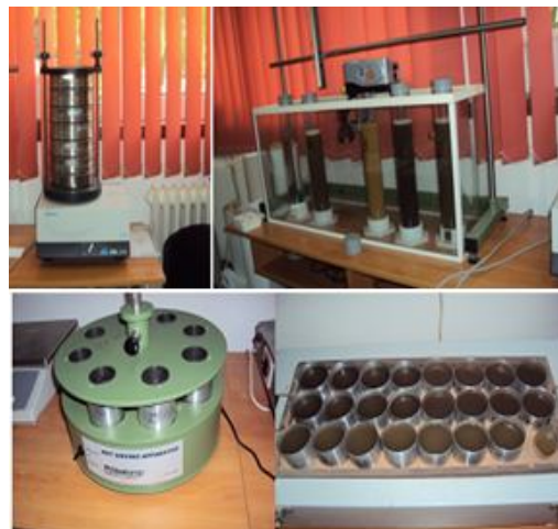
Figure 3. Sieving device and pipetting device . Device for determination the aggregates stability and sand box for drying
