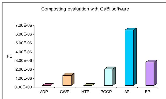
**Fig. 3** Environmental impacts generated by composting process determined with GaBi software
