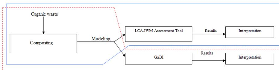
**Fig. 1** Schedule of evaluation of composting with LCA-IWM Assessment Tool and GaBi software
