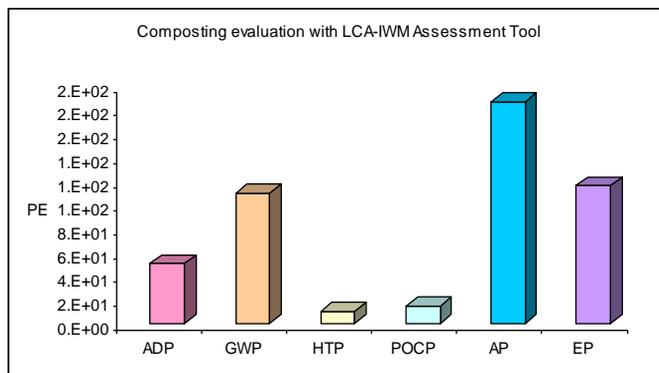
**Fig. 2** Environmental impacts generated by composting process determined with LCA-IWM Assessment Tool
