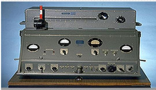
Figure 3 **Geodetic Distance Meter – NASM-2A built by swedish from AGA**
