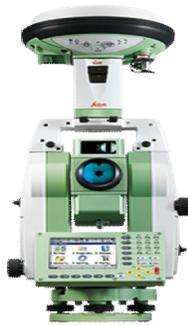
Figure 10 Leica Viva Smart Station
