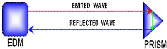
Figure 2 **Electronic Distance Measurement – EDM**
