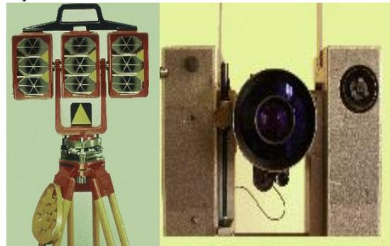
Figure 5 **Geodetic Distance Meter – Model 6 Geodimeter with battery of nine prisms**
