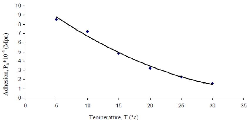
**Figure 2 - Experimental and predicted adhesion for saturated clay mud using quadratic polynomial as a function of temperature**
