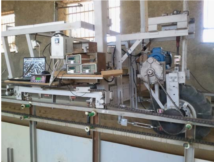
Figure 1 - Soil bin set up and its equipments
