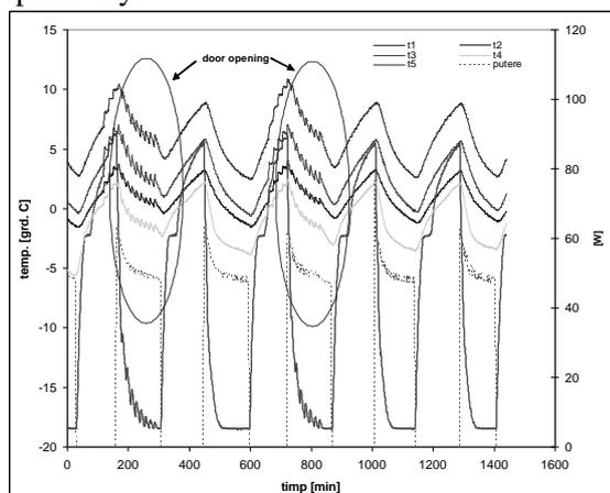
Figure 4 Energy consumption and temperature levels (10% load; with door opening; 25°C)
