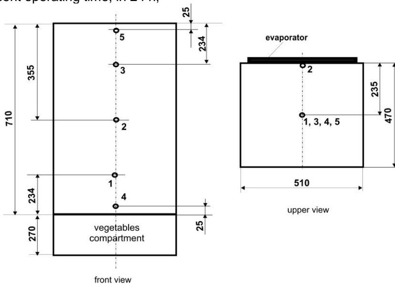
**Figure 1 Placement of the temperature probes**
