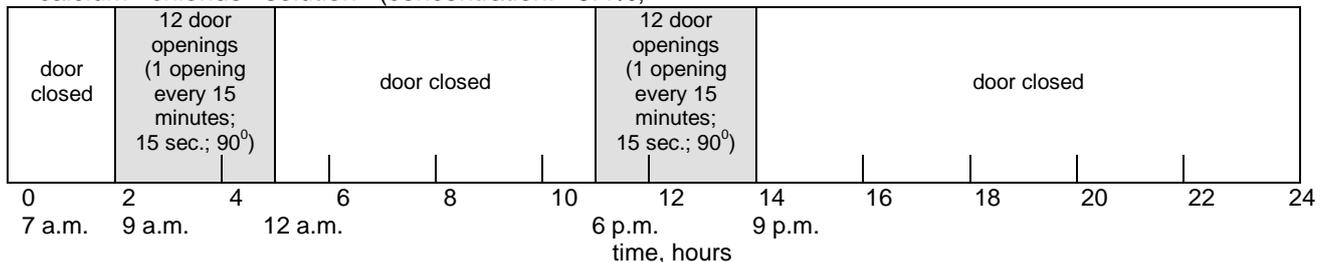
Figure 3 Test program with refrigerator door opening
