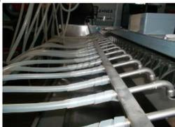
**Fig.2** Measuring ramp in the liquid leak position
