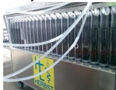
**Fig.3** Ramp with the liquid collector cylinders
