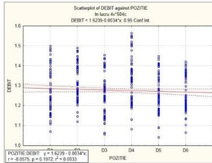
**Fig. 7** Influence of the position on the ramp on the average flow S/D
