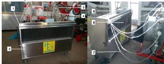
**Fig. 1** Stand for testing the distribution uniformity of the sprayers, Herbst ED 20-900
